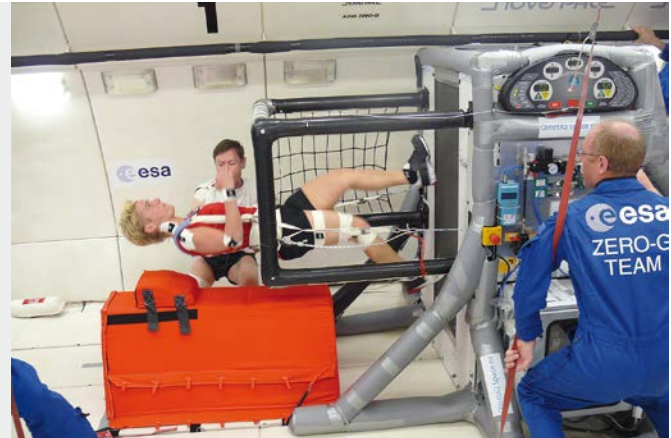
TUBUS are used to protect a fitness machine in zero gravity QinetiQ Space nv, 9150 Kruibeke, Belgium
